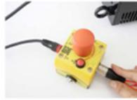
**C:** Insert the Remote Interlock Bypass to the E-STOP Remote to disable the interlock. (USA only)
