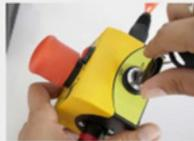
**B:** Turn the E-STOP Remote key to ON position.
