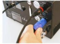
**D:** Use supplied Neutrik powerCON power cable to connect the laser system to a main power supply using the input connector.
