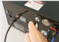
**A:** Turn the laser system key to ON position
